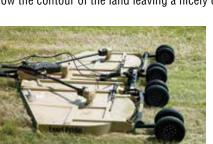
The 20' cutting width, 2" to 14" cutting height and ability to cut weeds and brush up to 3" in diameter make the RC5020 well suited for varied applications. Various safety guard choices make these an excellent choice for state and municipal mowing applications.
